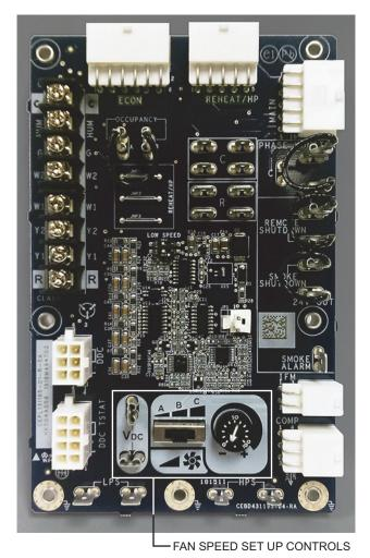
Fig. 7 — UCB Fan Speed Controls
