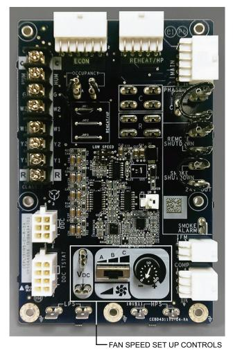
Fig. 47 — UCB Fan Speed Controls
