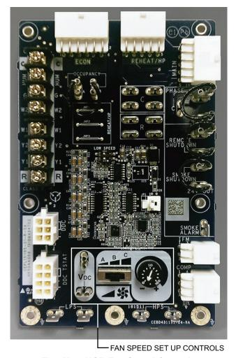
Fig. 48 — UCB Fan Speed Controls
